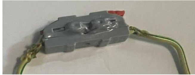
Fig. 5. Deformation of the E.NEXT p0660204 terminal block with a pressure lever following testing
