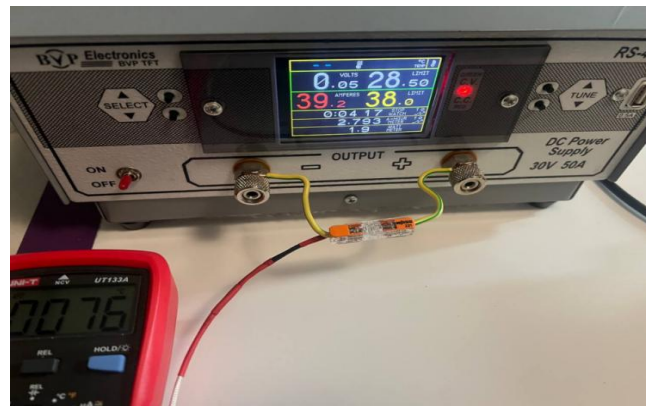
Fig. 6. Testing of the WAGO transparent 1-conductor terminal with lever 22-2611V-W
