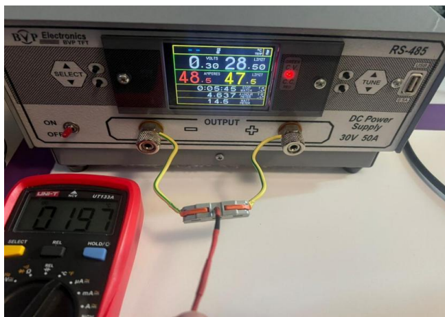
Fig. 3. Testing of the E.NEXT p0660204 terminal block
