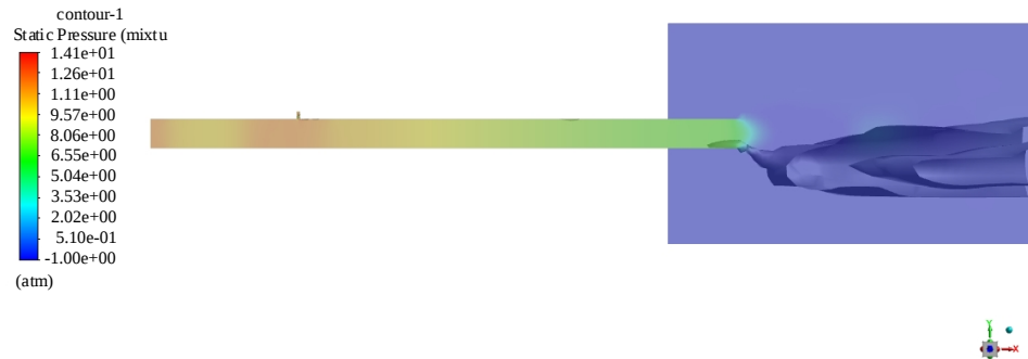
Fig. 8. Distribution of the liquid during the generation of a fine water-mist jet from the nozzle of the fire-extinguishing system under the action of shock waves at the simulation time of 5.11 ms
