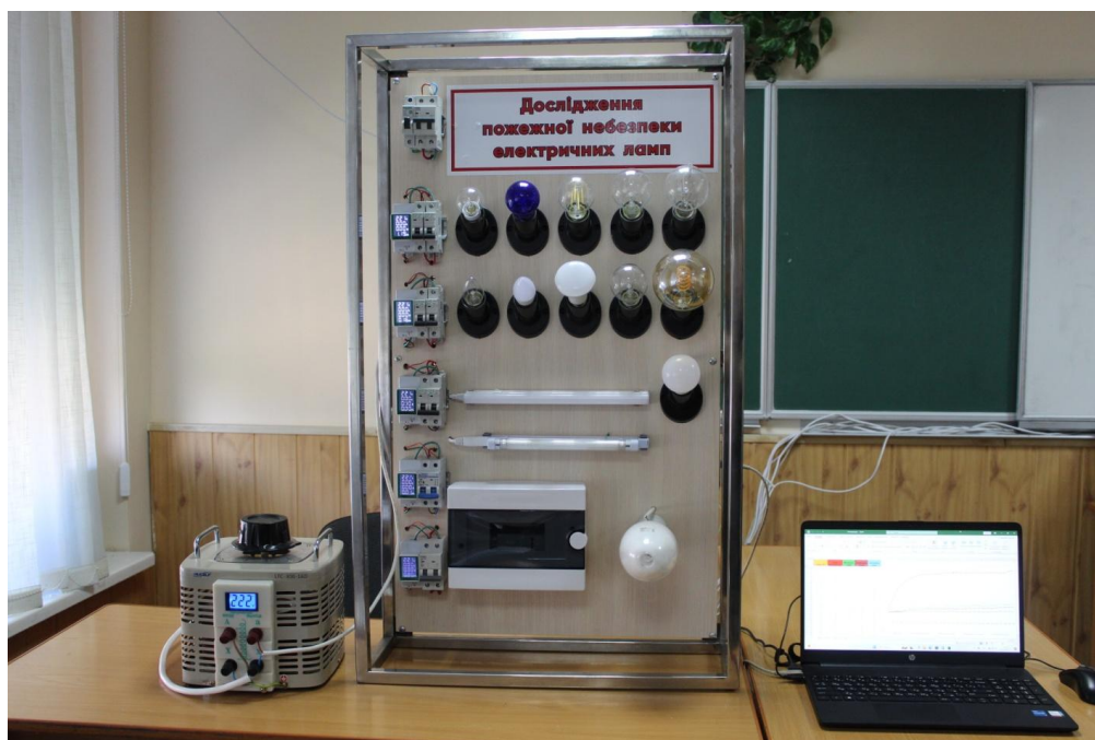
Fig. 1. Appearance of laboratory stand for fire hazard study of electric lamps
