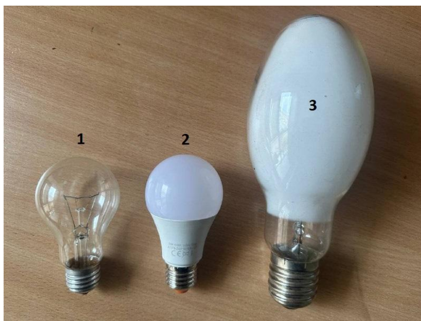
Fig. 2. Appearance of electric lamps of different types used for tests: 1 – incandescent lamp; 2 – LED lamp; 3 – arc mercury lamp
