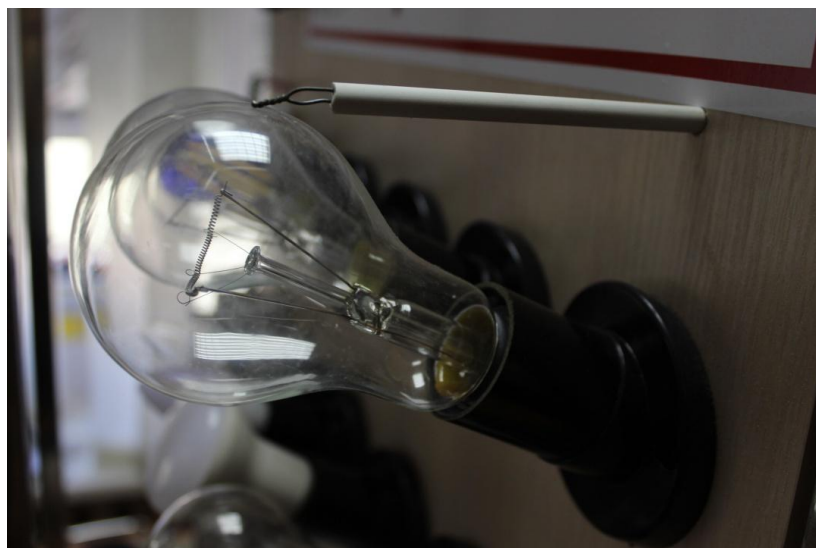
Fig. 3. Appearance of the thermocouple used to measure the temperature of the bulb of electric lamps
